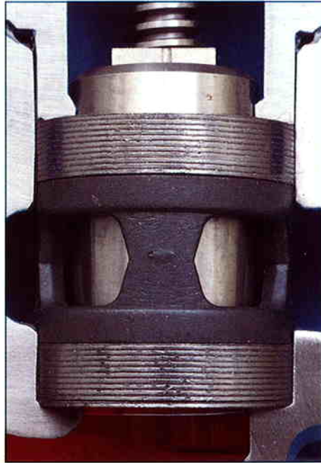
The bonnet (1) presses against the lower component with the sealing element. The two rings (2) and (3) are pre-sealed and increase their coupling pressure on the casing and piston.
